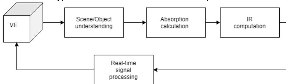
Fig. 1: a diagram showing a design for the system proposed. a method for object/scene understanding is applied in order to extract information that would be used to calculate sound absorption of surfaces and objects. As a result, impulse responses would be computed and integrated to the sound signal through real-time algorithms.
