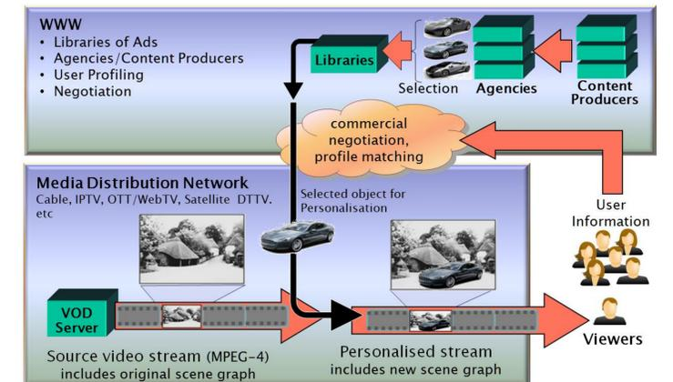
Above – The general principle of inserting a selected object from a network library into a playout stream; the selected object personalizes the video image for the specific user.
