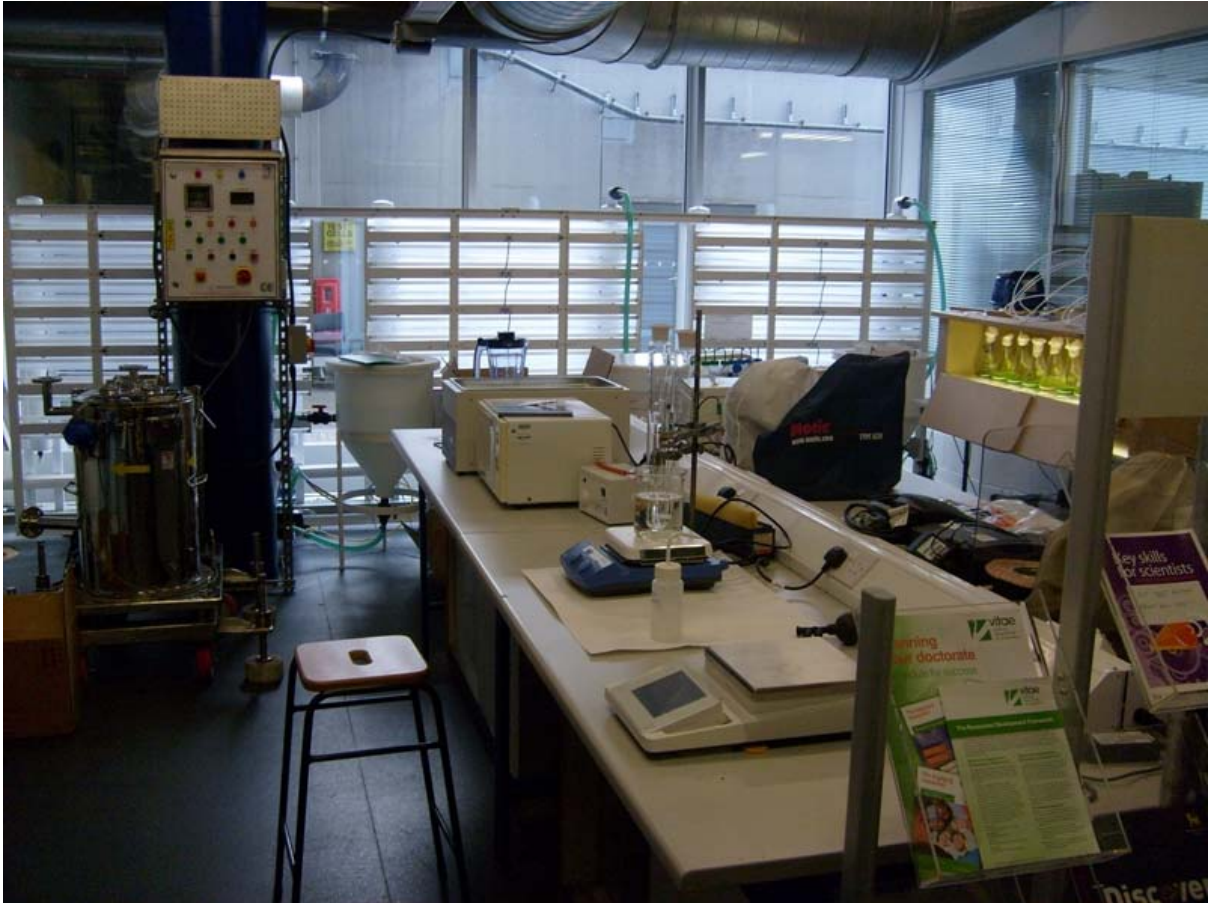
Figure 3. Showing Bioenergy lab, note three photobioreactors (PBR's) culturing microalgae just before the window.
