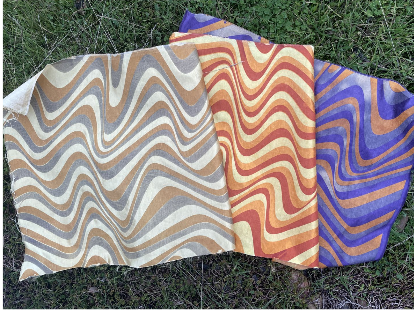
Colours and 3 colour prints developed using pomegranate, sappanwood, madder and coreopsis, modified with iron, copper and citric acid.
