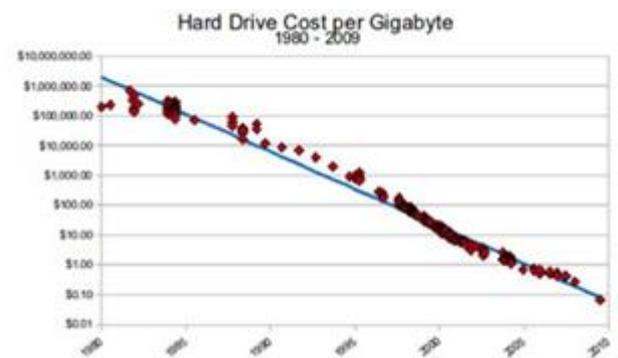
Fig. 20: Cost of hard drives per gigabyte. (Labourey, 2012)
